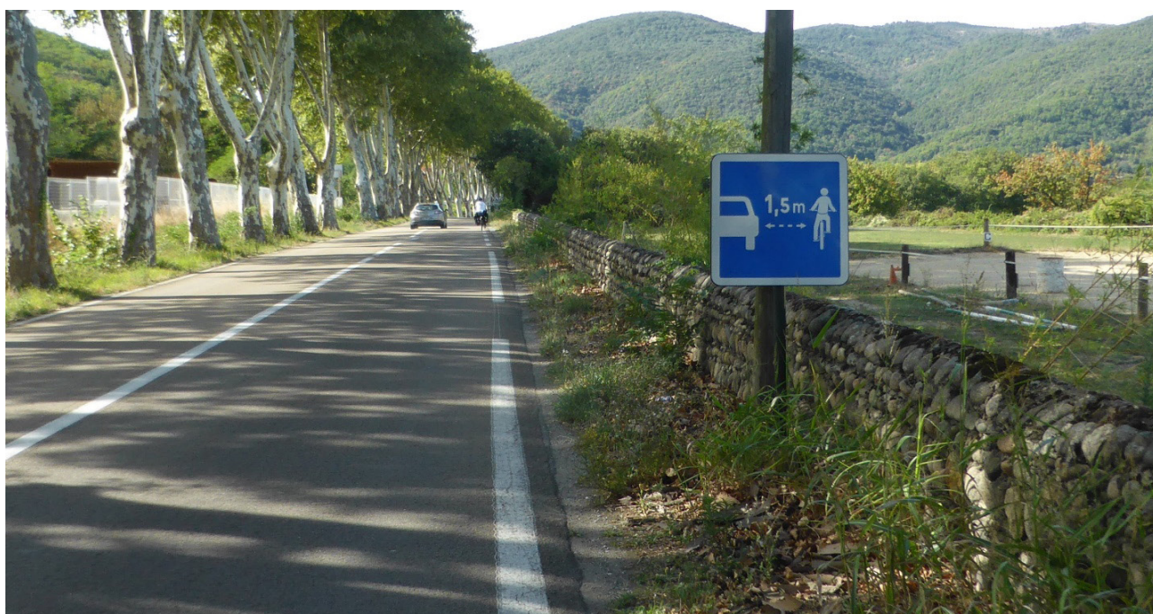
Example (from France) of a sign for drivers indicating the minimum distance to cyclists that needs to be observed when overtaking.
