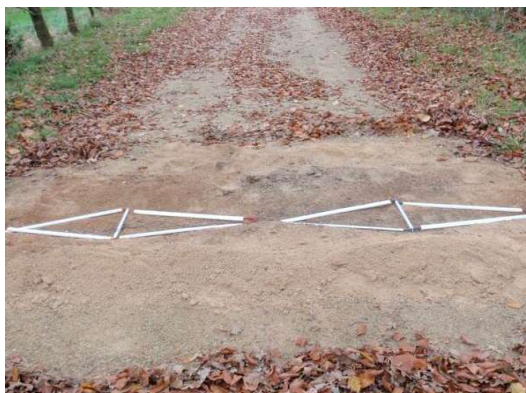
Figure 2 Inductive loops on natural soil, source: Eco-counter
